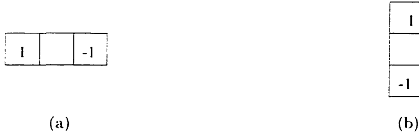
Figure 3.11 Example of differential masks (a) in x -direction and (b) y -direction.
